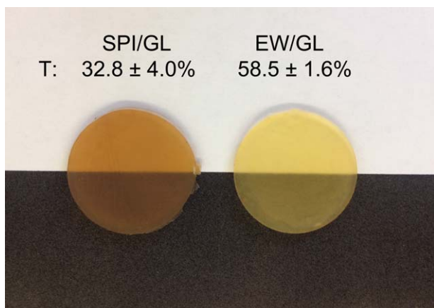
Figure 7. Physical appearance of SPI/GL (left) and EW/GL (right) bioplastics processed through injection molding, respectively, an injection pressure of 500 and 600 bars, respectively, and a molding temperature equals to 120°C, for both of them. Transmittance ( T ) was obtained at 600 nm. [Color figure can be viewed in the online issue, which is available at wileyonlinelibrary.com .]
